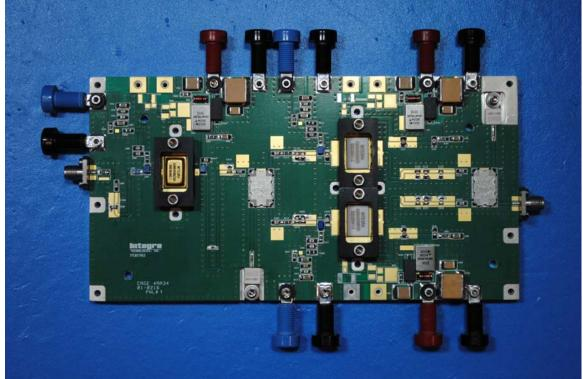
IGNP0450M1000 operates over the frequency band of 420-450 MHz. Under 100us – 10% pulse conditions, it supplies typically 1 kW of output power with 75% power added efficiency and 42 dB gain from a 75V supply voltage across the case temperature range from -25°C to +85°C. It weighs only 350 gr. and it's smaller than today's tablets.
